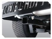
Hitch Receiver – Class 1 hitch for easier mounting of accessories
