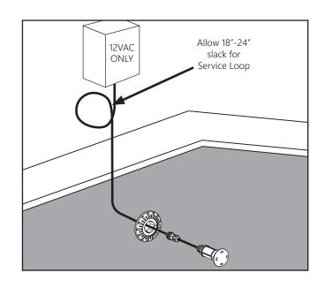
An example of an approved pool transformer is the Intermatic model PX-100 or PX-300. Refer to Wire Gauge and Wire Length guide for proper wire gauge size in reference to the use of Junction Box installations.
