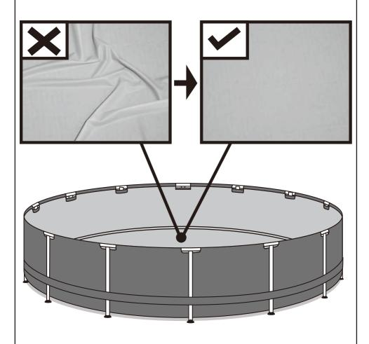
Put 1 in. to 2 in. water in the pool to cover the floor. Once pool floor is slightly covered, gently smooth out all wrinkles. Start in the center of the pool and work your way clockwise to the outside.
