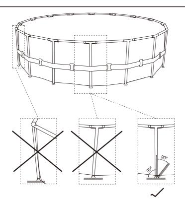
After the installation of the pool's steel frame is completed, ensure that the verticals are perpendicular to the ground. If they aren't, the verticals could be bent or deformed.
