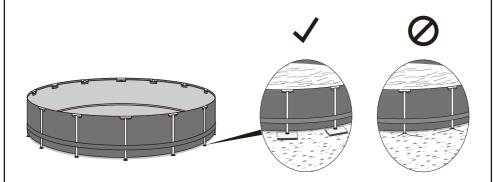
Do not assemble with pool legs on soft lawn. If you must assemble the pool on a soft surface, timber boards (not included) must be placed under the feet of the vertical support rods for even weight distribution.
