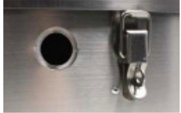
Remove the nut from the photo cell & unplug the jumper connection from the transformer.
