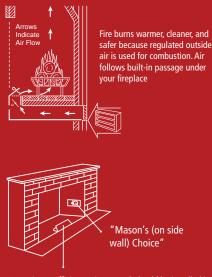
For optimum efficiency Air-A-Lator $^{\otimes}$  should be installed in the front row of brick in center of fireplace with opening facing fire or grate.
