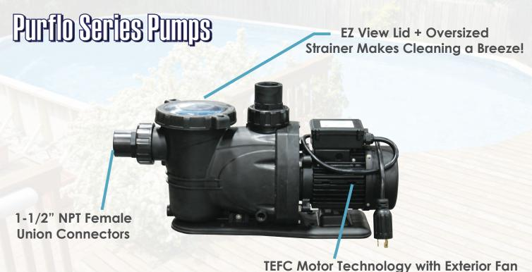
for Efficient Motor Cooling
