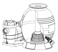
4. Insert the tube with the diffuser body inside the tank as above picture, then place the funnel on the tank's mouth and pour 45lbs of the No. 20 Silica Sand with particle size of 0.45 mm-0.55mm sand into the tank
