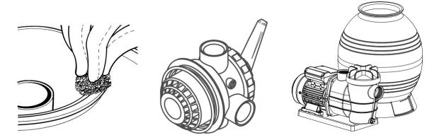
6. Connect the sand tank to pump with hose, hose clamps and hose adaptors.
