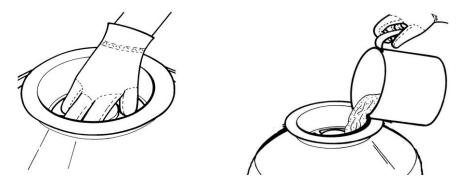
5. Take away the funnel, and then clean really carefully the tank's neck and fix the valve with O-ring through flange clamp set. (the direction of "PUMP" port on valve needs to face pump out port)
