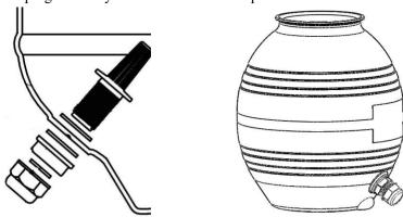
3. Press and turn the sand tank to mount it to sand filter support with correction direction (drain plug is at outside as below picture).
