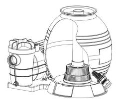
4. Insert the tube with the diffuser body inside the tank as above picture, then place the funnel on the tank's mouth and pour 45lbs of the No. 20 Silica Sand with particle size of 0.45 mm-0.55mm sand into the tank
