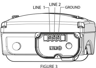
Note: If GFCI circuit breaker protection is required, the pump should be ground wired on its own independent circuit. AquaStar Pool Products recommends using a Siemens Class A Double Ground Fault Circuit Interrupter.
