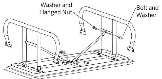
8. Locate one of the Seats and position it up to the Support Seat Brackets. Line up the mounting holes in the Seat with the mounting holes in the Support Seat Bracket. Insert a Bolt with Washer through the each of the sets of mounting holes and tighten finger tight.
