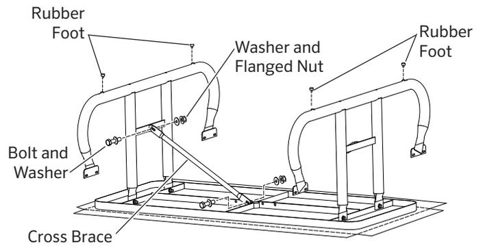
7. Attach the other Cross Brace to the Tabletop and other Support Bracket in the same manner. Leave the hardware finger tight.
