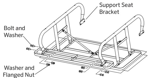
9. Turn the table right side up and tighten all hardware while checking with a Level.
