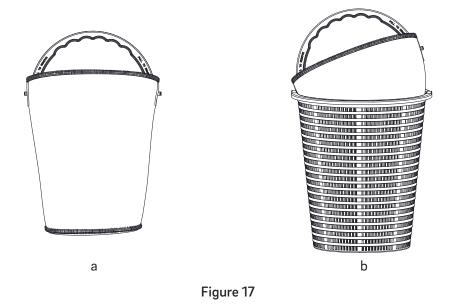
4. To reinstall the silt-sock into the basket, locate the manufactured holes in the silt-sock and push the handle pins into each hole and then begin by inserting the pins into the basket (Figure 17b). Once complete, roll the silt-sock over the basket lip (Figure 18a).
