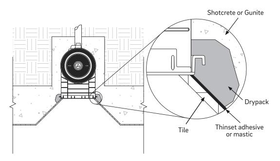
5. Once the shotcrete is complete, cut the capped pipe that was installed on the venturi discharge line (Figure 3) so that it will be flush with the finished surface. Add glue to the pipe and slide a waterstop (Figure 9c) over the pipe, allowing enough room to dry-pack behind it to ensure a waterproof seal (Figure 8).
