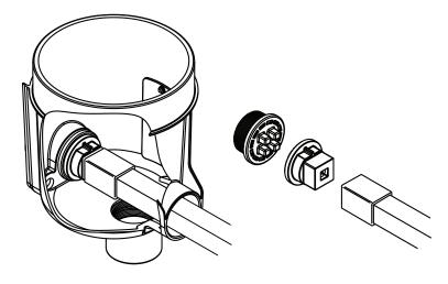
7. After applying the finished surface, install the QuikGuard "knock-In" wall fitting (Figure 13a) and remove the weir door guard (Figure 13b). Install weir at startup.
