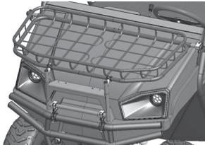
Using a #4 allen wrench and 10mm wrench, attach the two rear clamps (E) to the ROPS clamp (F) with two M6 x 20mm button head bolts, 4 washers and 2 nuts as
