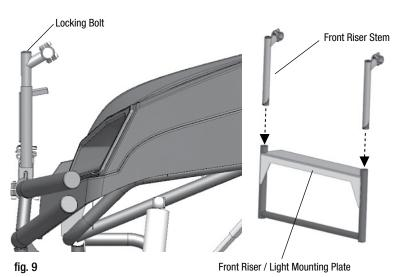
Adjust the width of the extendable tubes (G) so they stick out just past the clamps as shown below. The hood rack angle can be adjusted by loosening the bolt on the front riser stems and lifting up or pushing down on the front of the rack. Adjust clamps and brackets as necessary, then tighten all bolts. We recommend no more than 5% of slope to the hood rack.
