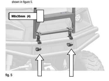
Place the 2 ROPS clamps (E) approximately 6.5" up from the top of the mud guard as shown in figure 6.
