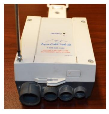
**PUT COVER ON AND REINSTALL SCREWS**
