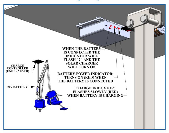
Once the solar charger has been installed, and a battery is installed onto the lift the 24V Solar Charger will turn on and start trickle-charging the battery. Without the battery installed the 24V Solar Charger will be off, and will remain off until a battery is installed.
