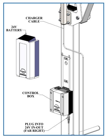
NOTE: Make sure the plug is fully engaged into the control box. Make sure the lights come on (see next page) and the lift functions normally when the 24V Solar Charger is installed. If the lift does not function, check all connections going into the control box and make sure they are pressed all the way in. When installed properly the battery will charge as the lift operates simultaneously.
