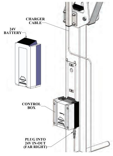
NOTE: Make sure the plug is fully engaged into the control box. Make sure the lights come on (see next page) and the lift functions normally when the 24V Solar Charger is installed. If the lift does not function, check all connections going into the control box and make sure they are pressed all the way in. When installed properly the battery will charge as the lift operates simultaneously.
