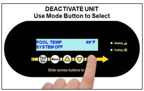
Select the pool or spa thermostat. Then press the up or down arrow to set a desired temperature (set point) for the water.
